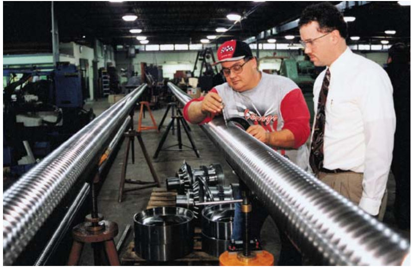
Wedin has produced the world's largest ball screw assemblies at over 50 feet in length.
